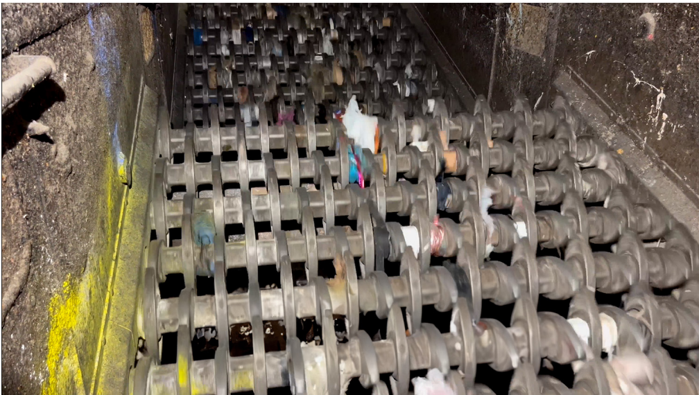
Glass is separated when it breaks and falls through the gaps of the sorting screen discs.
